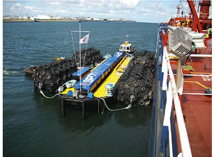
SPT1 is our latest lightering support vessel operating out of Rotterdam Europoort - a pontoon boat that has been converted to store all the required equipment for STS operations, enabling SPT to have all of the equipment in one location.
