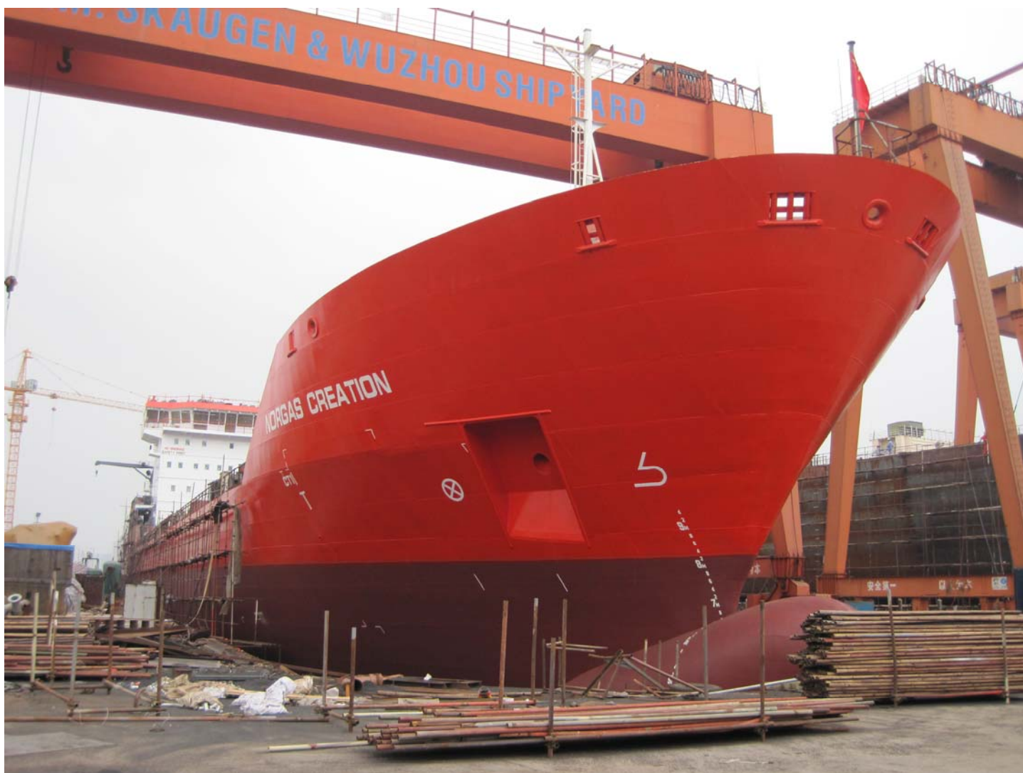
The Norgas Creation – second Multigas-vessel of a series of 6 and under outfitting stage as being completed by Skaugen Marine Construction in China (SMC). The ship is an advanced LNG/ LPG/ Eth gas carrier – 10 000 cbm
