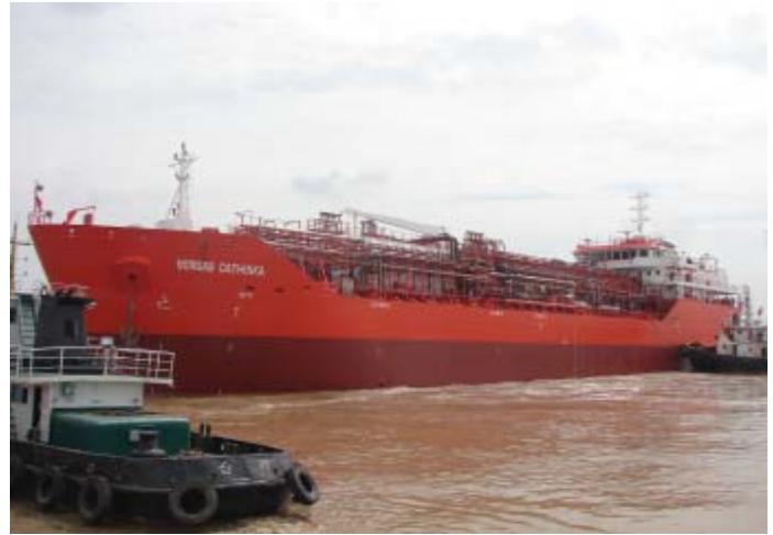
Norgas Cathinka – 2nd Wintergas vessel to be delivered in the end of October 2009. The ship is a Special. LPG/Eth/Chemical combo carrier – 5 800/ 9 600cbm.
