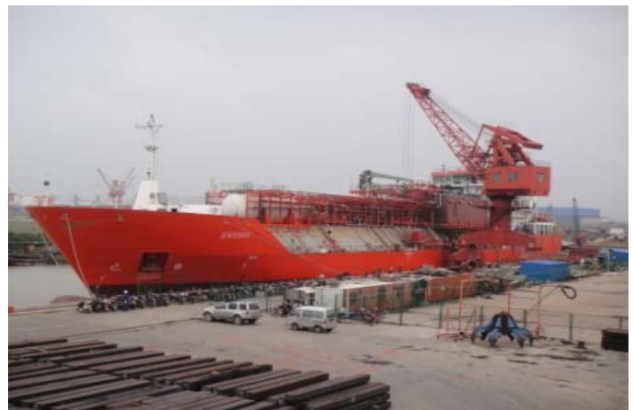
Norgas Innovation – 1 st Multigas vessel is under final outfitting. The ship is an advanced LNG/ LPG/ Eth gas carrier – 10 000 cbm.
